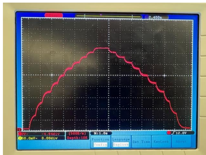
Figure 18 - Oscilloscope Capture when adjusting the duty cycle from 0% to 100%
