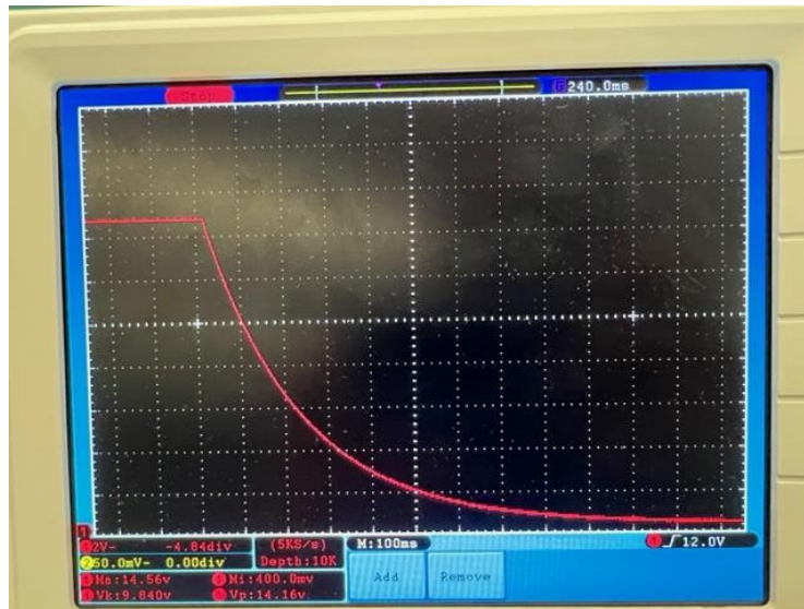
Figure 22 - Oscilloscope capture ramp down of the power supply
