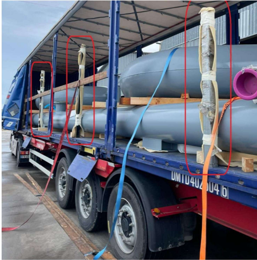
Figure 14 – Example of Loaded Pipe Lorry showing dunnage beneath assemblies creating localised patch loads on the deck. Source: REN Group Document IS.STD.060
