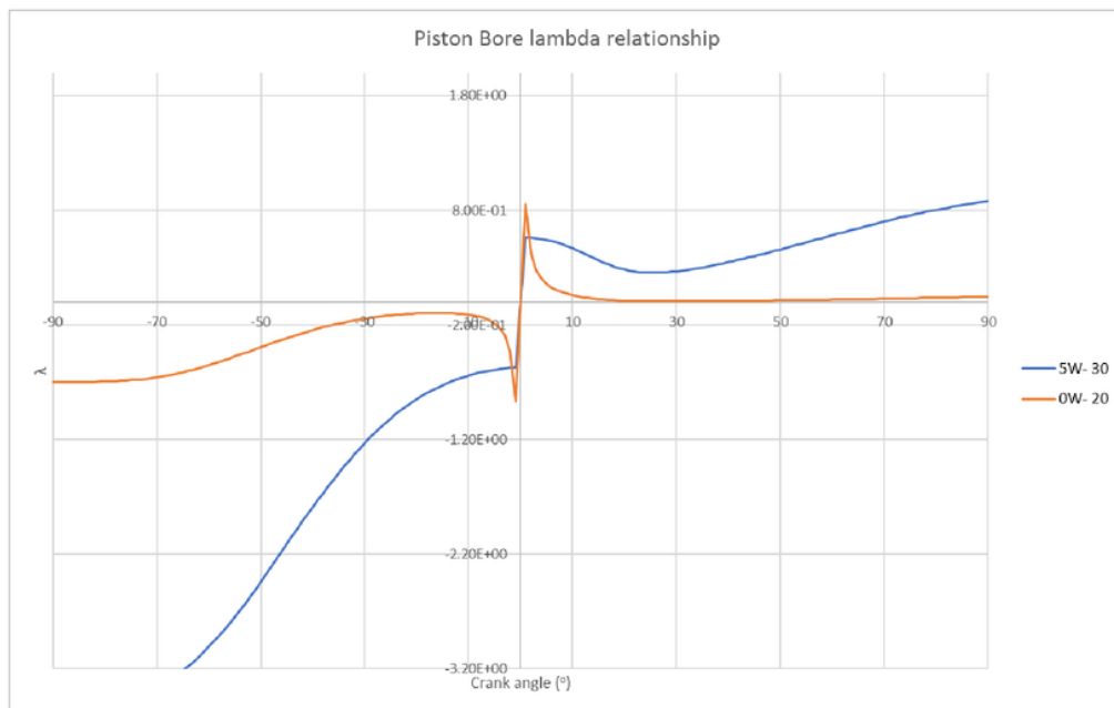
Figure 24 - Piston bore lambda value of standard inline crank geometry with respect to different viscosity lubrication.
