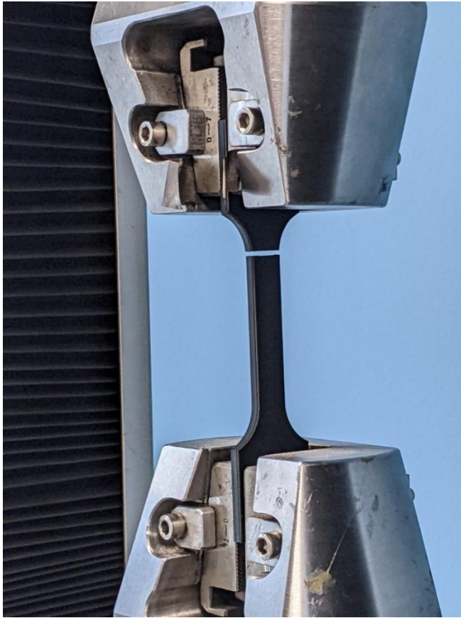
Figure 22 Image of a fracture in an out-of-plane billet sample
