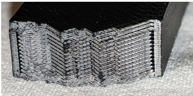
Figure 25 Image of 'bias' fracture section
