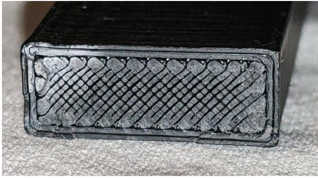
Figure 23 Image of out-of-plane fracture section
