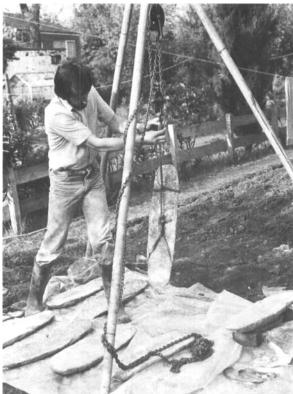
Figure 3. Photograph showing possible purpose of cuts in sides to assist in handling ingots.
