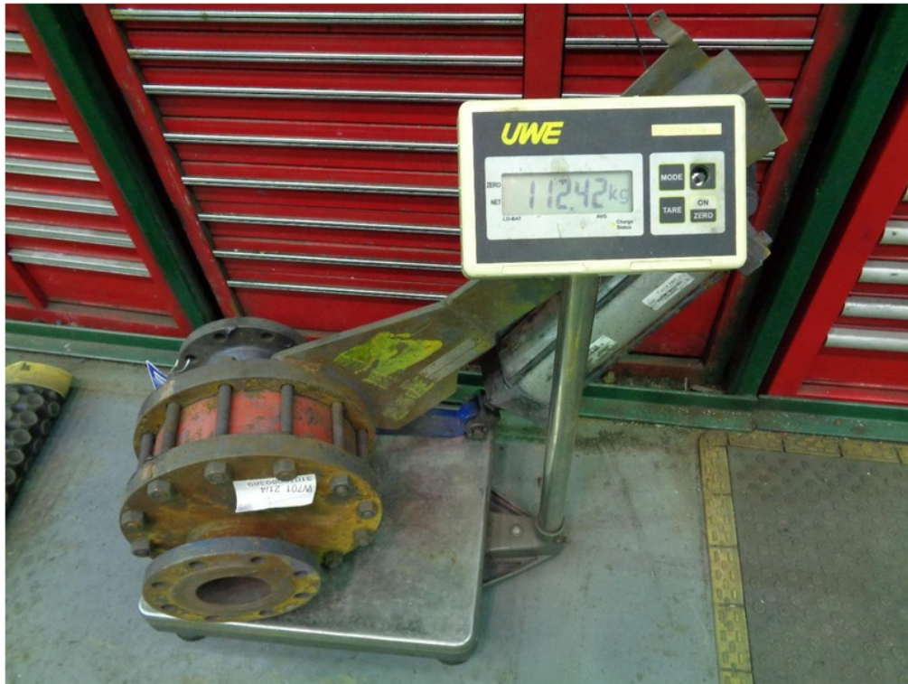
Appendix 1.4 – Wear on lever arm shaft that causes valve failures
