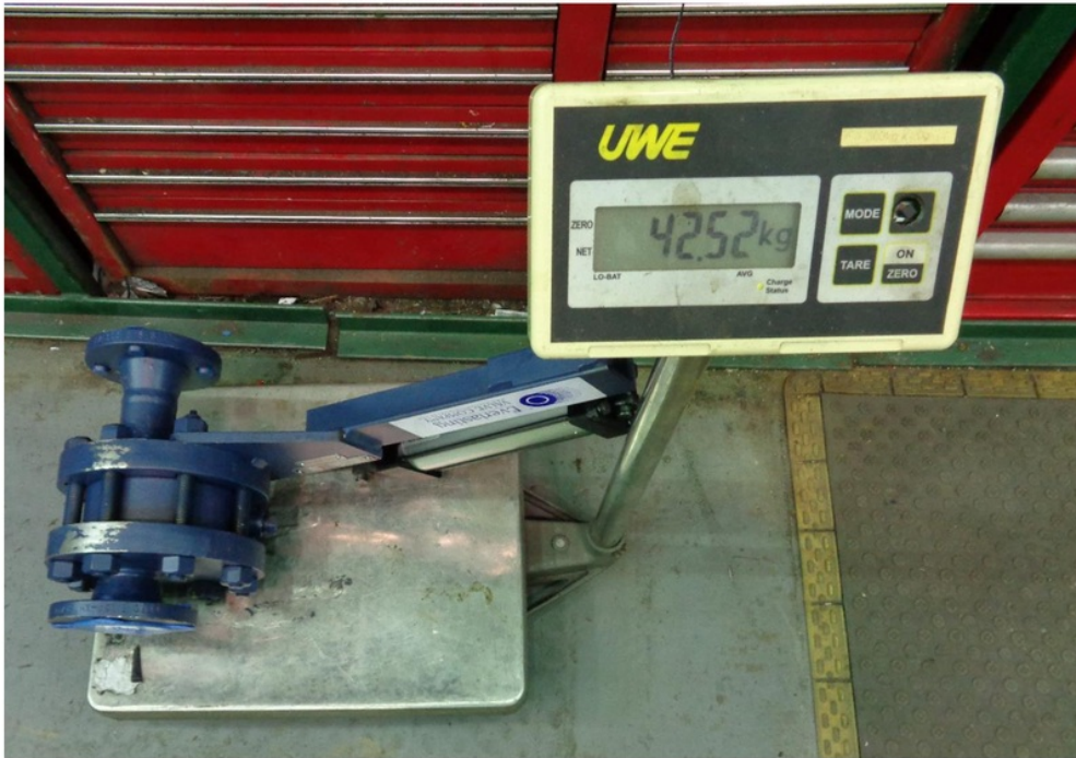
Appendix 4.1 – Weight of 2" Everlasting valve before installation
