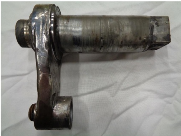
Appendix 1.4 – Wear on lever arm shaft that causes valve failures
