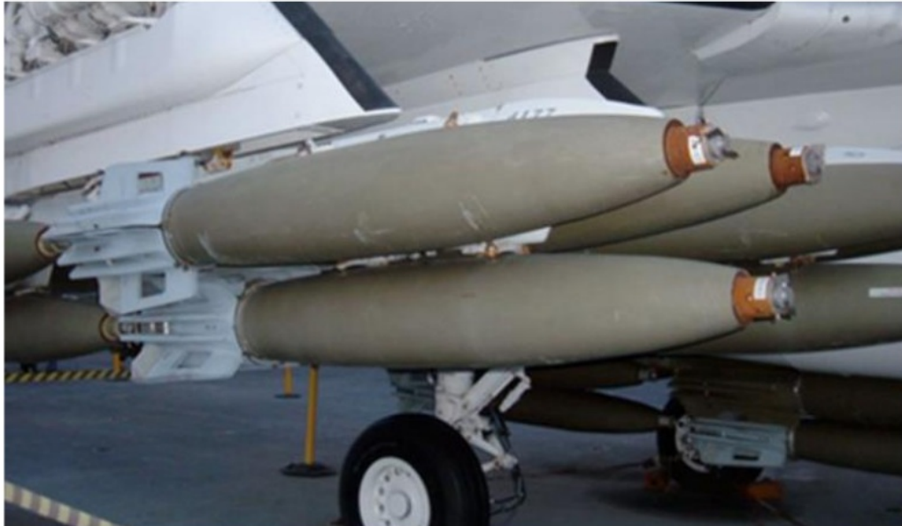
Figure 1 - Mk 82 type aircraft bombs fuze and fitted to an A-6 Intruder (photo credit: © BrokenSphere / Wikimedia Commons) [1]
