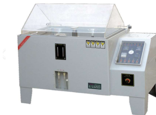
Image of a salt spray chamber. (Tensionmachine.com, 2023)
