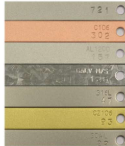
Image of corrosion testing coupons. (IndiaMart, 2023)
