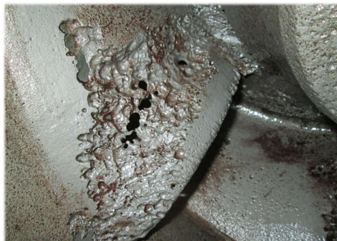
Image of an impeller that has suffered severe cavitation. (Detloff.C, 2021)
