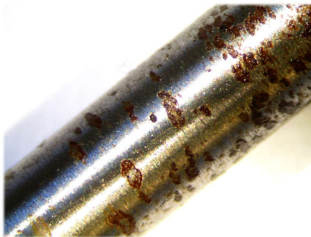
Image of metallic pipe with visible pitting ( ResearchGate.net, 2015 )
