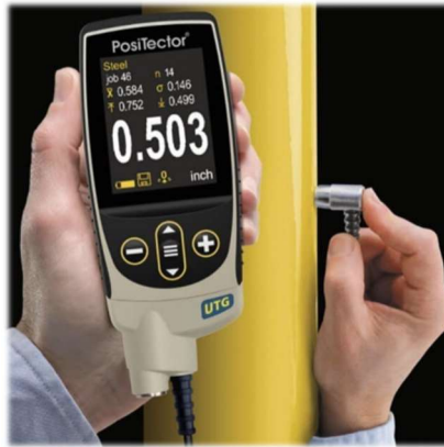
Image illustrating the use of a material thickness gauge. (ElektroPhysik, 2023)
