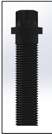
Figure 24 Standard Con-Rod Bolt Solid Works Model
