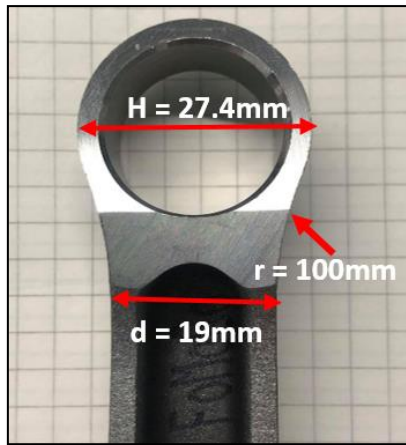
Figure 11 Con-Rod Point A Stress Concentration
