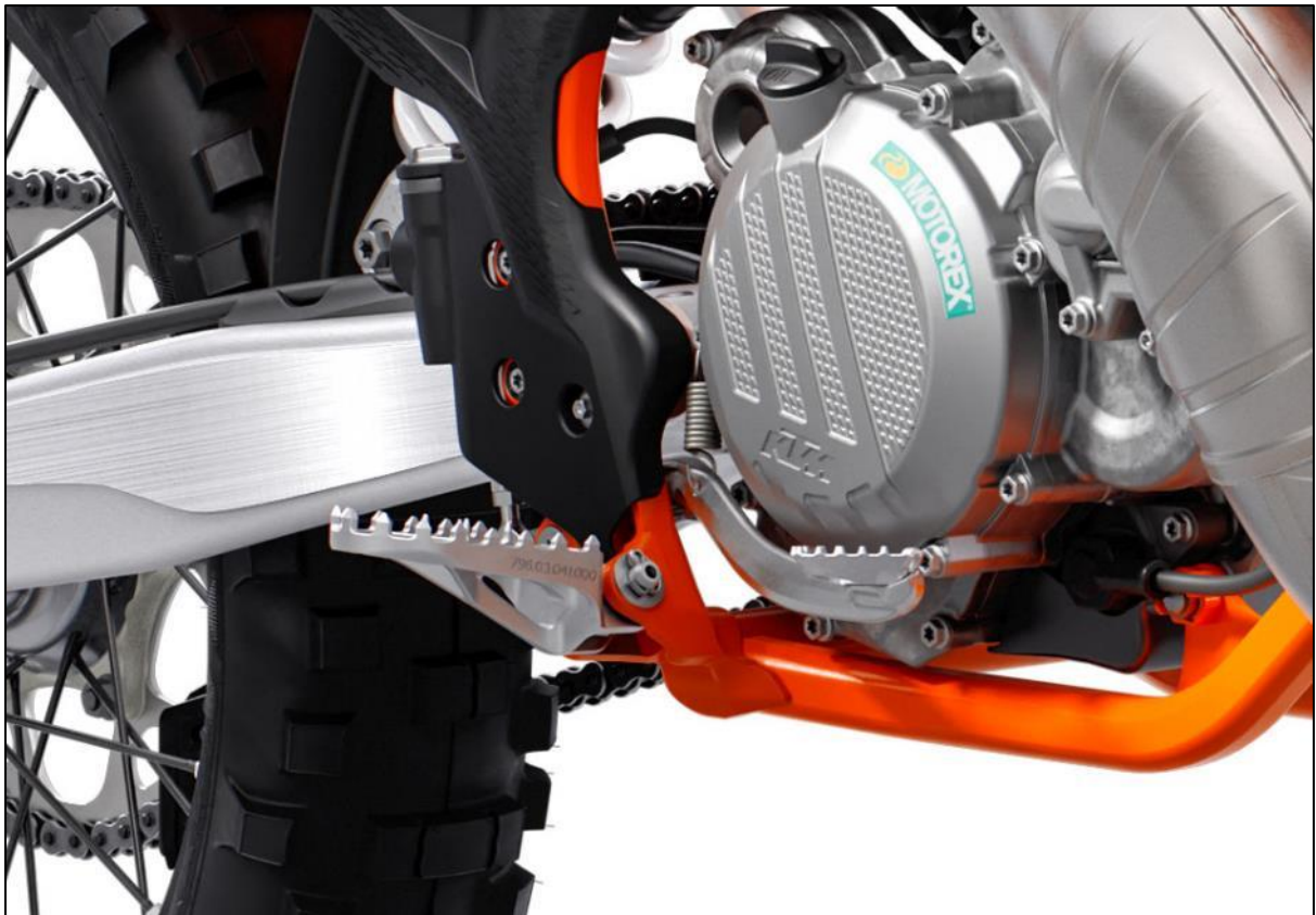
Figure 20: Original footpeg on a KTM EXC 300 motorcycle (KTM Malaysia, 2024)
