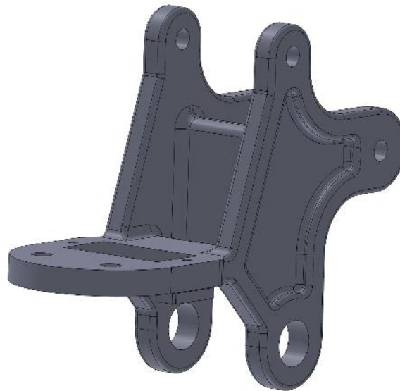
Figure 16: 3D model of revised robot gripper housing.
