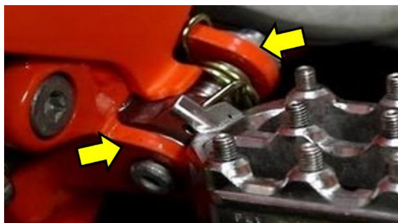
Figure 32: Motorcycle foot peg mounting points (Supermotodaz, 2024).
