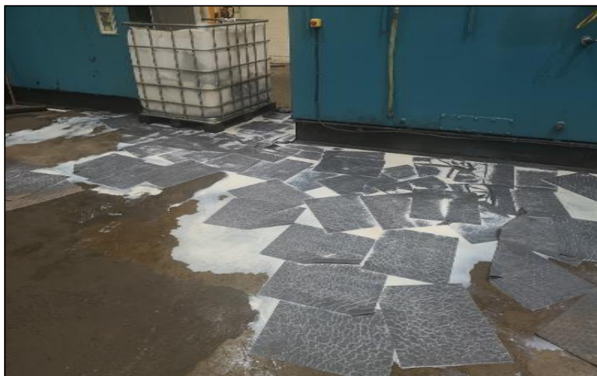
Figure 2: Hoffman Filtration Typical Breakdown and Coolant Overflow Event
