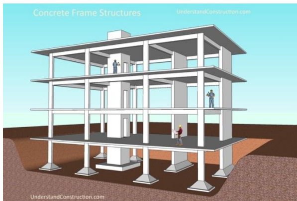
Figure 2 – Concrete frame diagram (Construction, n.d.)
