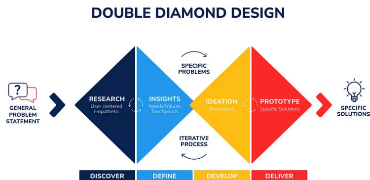
Fig. 1 - The Double Diamond design methodology
