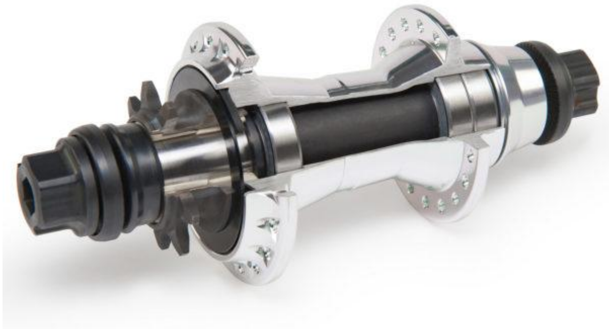
Figure 4: Cutaway of cassette hub
