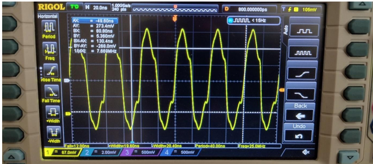
Figure 5 An image of an oscilloscope probing a 25MHz signal
