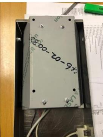
New PCB cover introduced to protect against steam/ humidity
