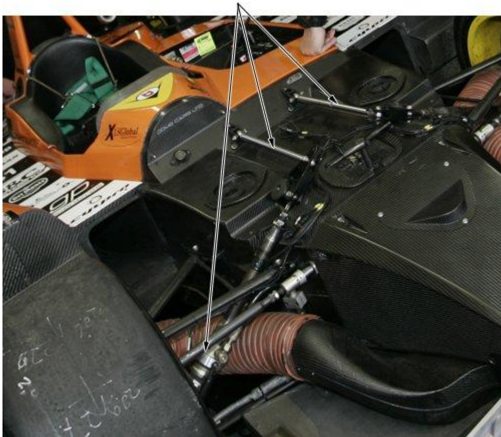
New hydraulic system. The coilovers have been removed and replaced with solid bars to prevent movement. The hydraulic units are on the bottom of the pushrods close to the wheel.
