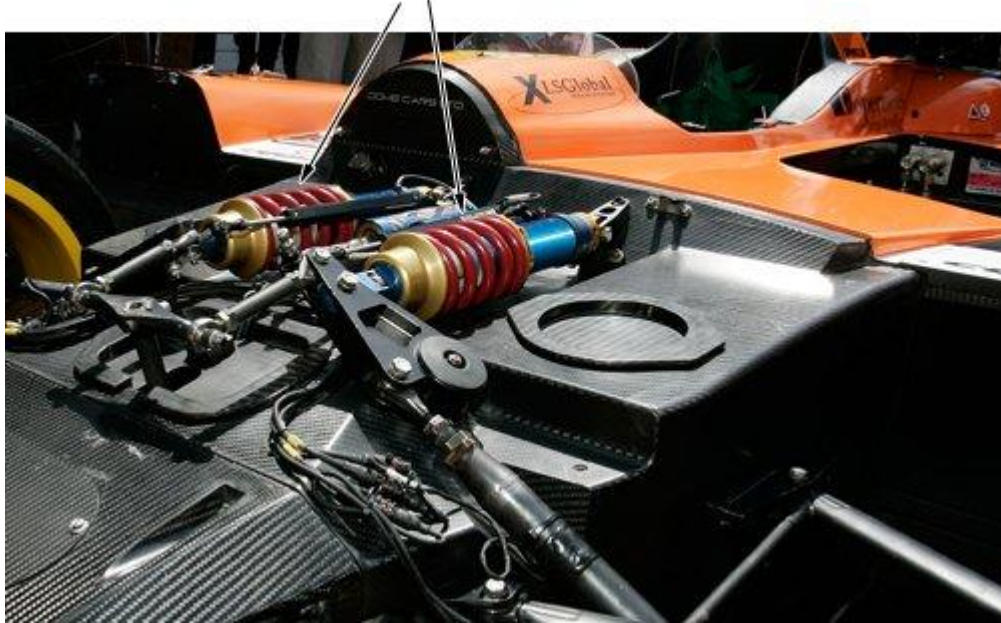
Traditional front suspension using coilover units
