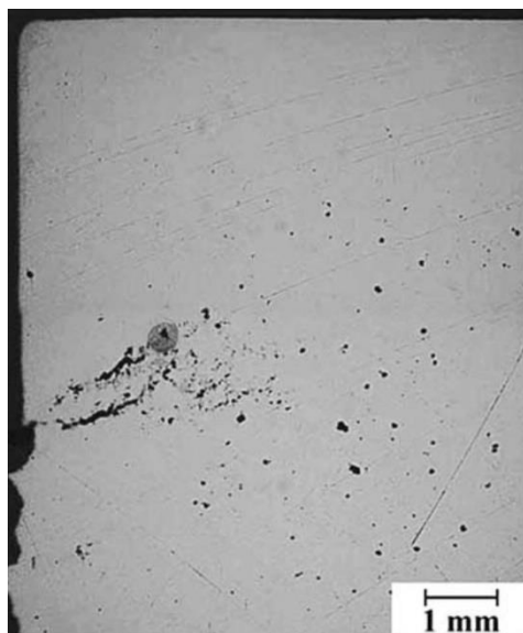
Figure 8 Fractures in Cast Aluminium due to cooling during shrinking. (S Otarawanna, 2009)
