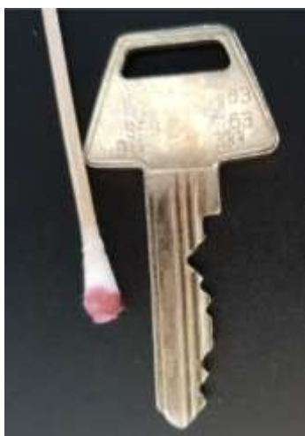
Figure 3 - Positive DMG test reaction as indicated by colour change
