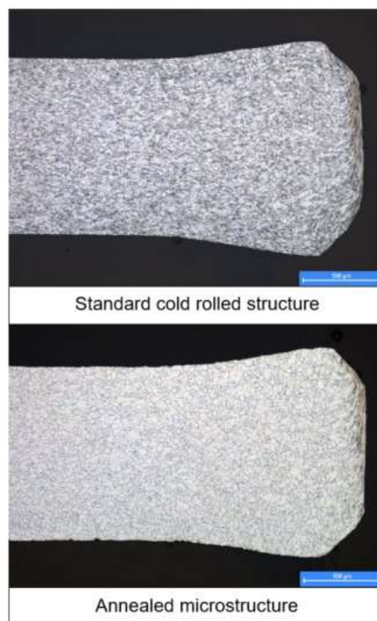
Figure 1 - As rolled and as annealed microstructure of mild steel blank
