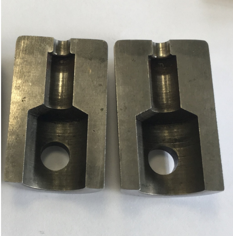
Figure 17 new set of collets for the Hounsfield. (Fadul, 2018)
