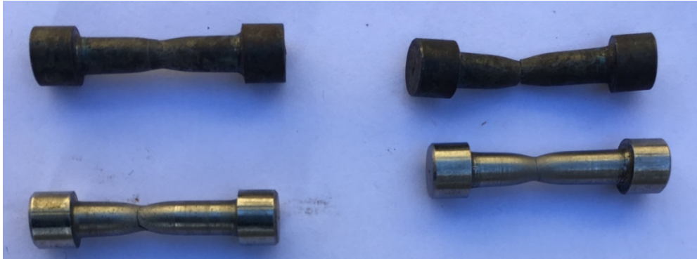
Figure 24 specimens after changing the collets. (Fadul, 2018)
