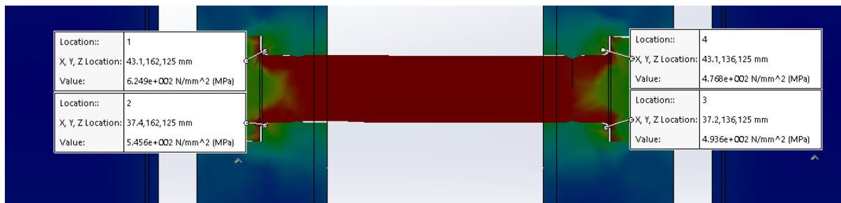
Figure 43 Stress plot for Denison final jig.
