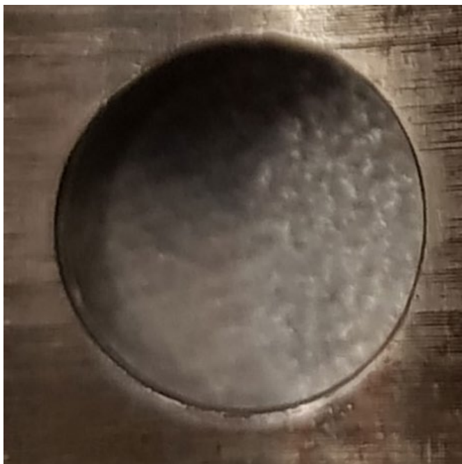
Figure 1 one of the two collets which make up the Hounsfield jig. (Better condition)
