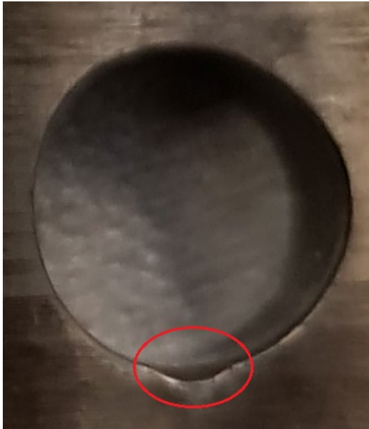
Figure 2 the second collet which makes up the Hounsfield jig. (Worse condition)
