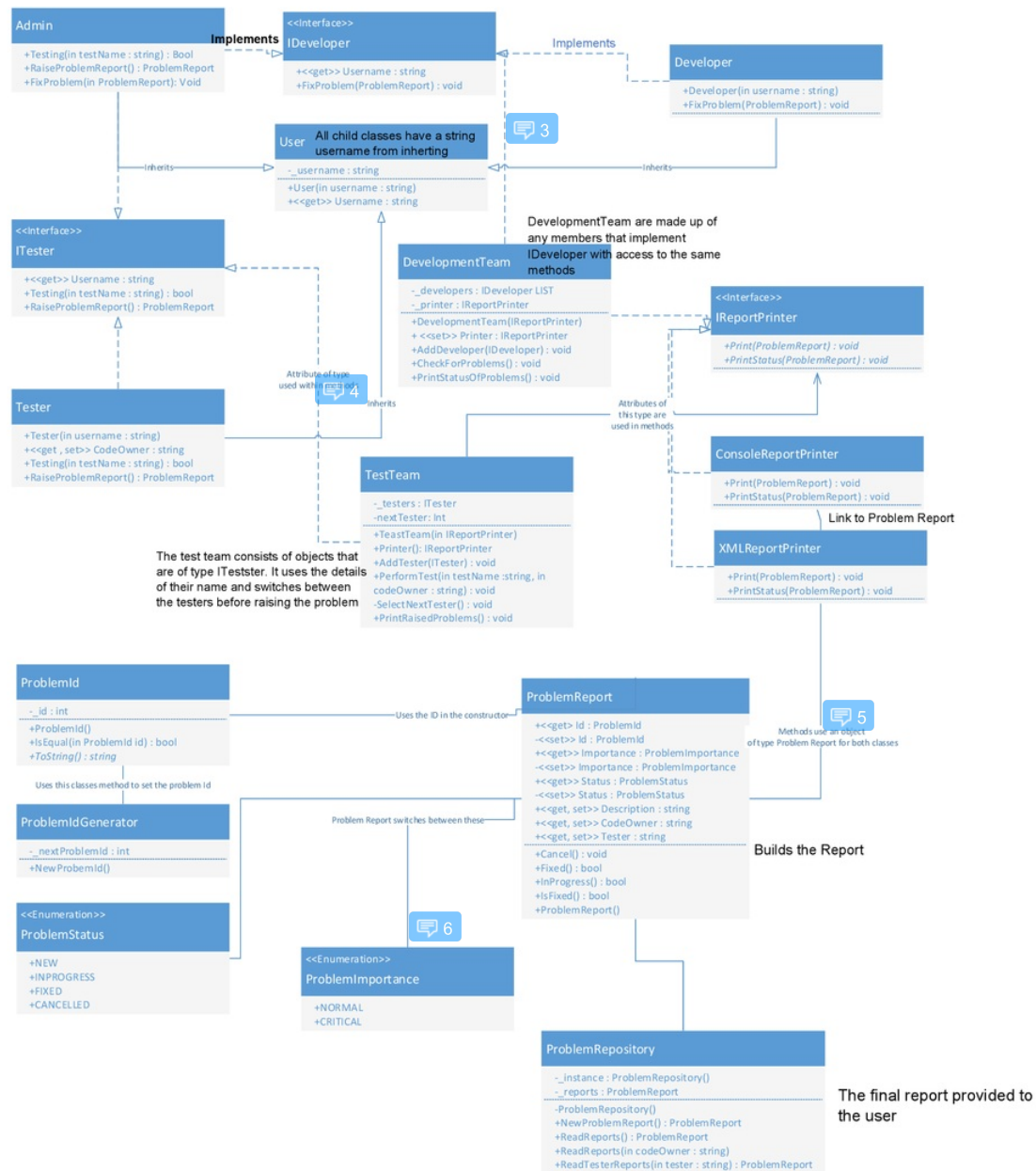
Fig 11. Class diagram for the program provided.
