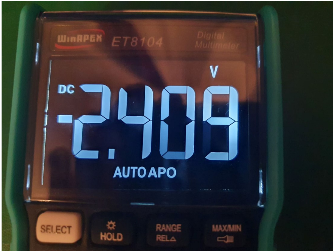
Figure 5.16 – Troubleshooting: real-time clock voltage reading
