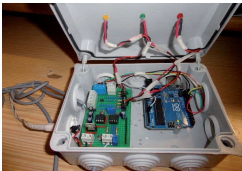
Figure 2.1 - Terrarium control system by [12]
