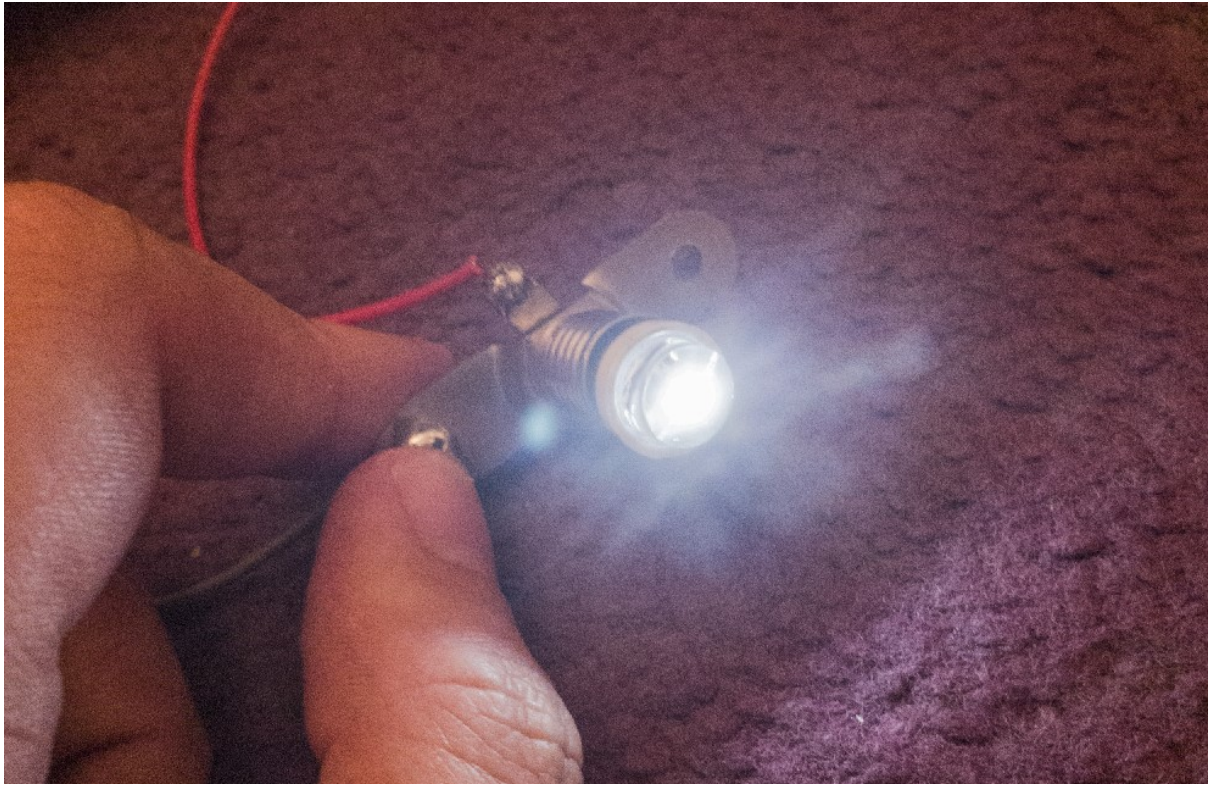
Figure F-7 – LED light as a replacement for a heating lamp, due to time constraints
