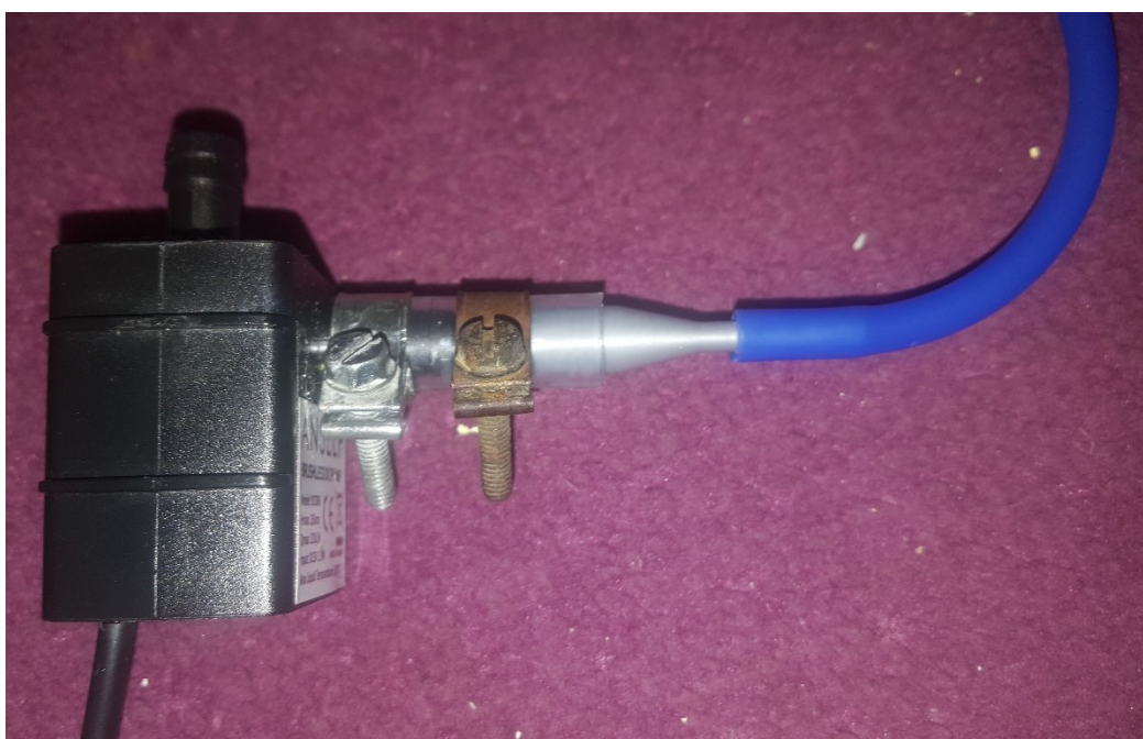
Figure F-6 – 3D printed pump tube adapter
