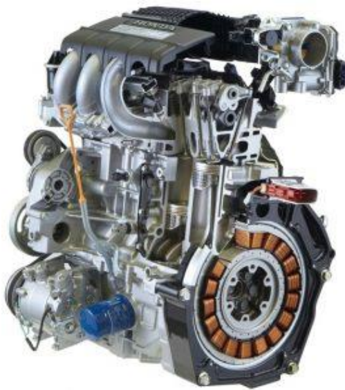
Figure 11 Shows an Integrated Motor Assist (IMA) with a single clutch for a mild hybrid produced by Honda (x-engineer).
