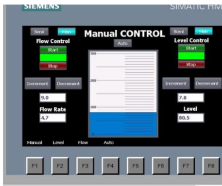
Figure 6 -manual control screen
