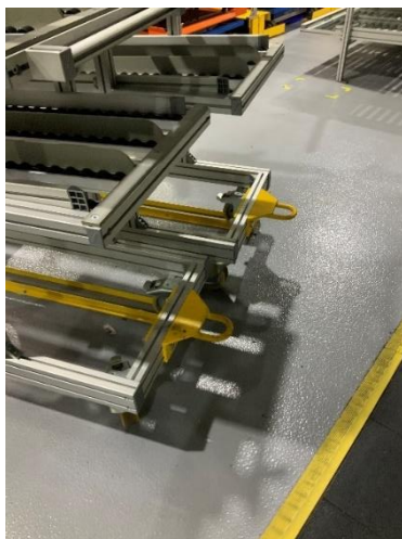
Figure 5 - CTDA trolley tow point
