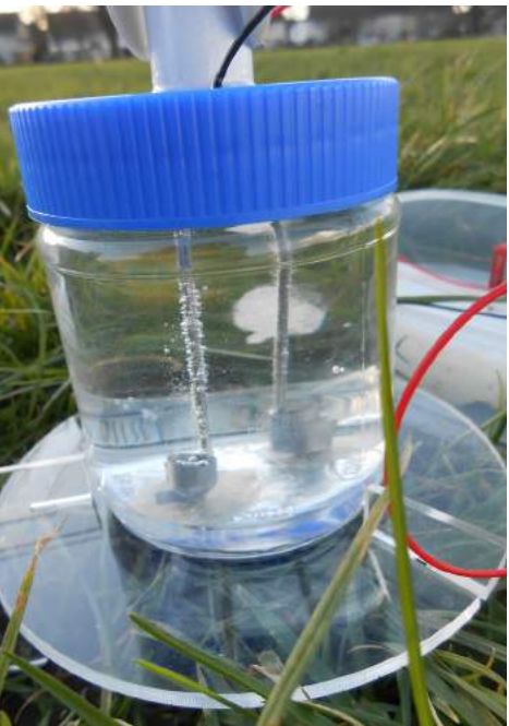
Early prototype testing (adjusting electrodes and igniter position)
