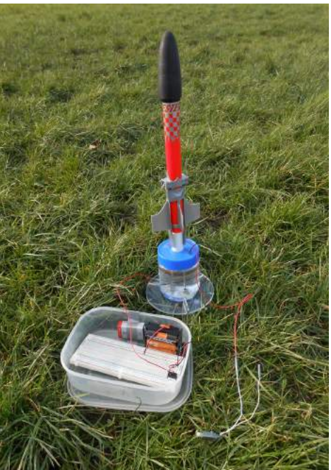
Early prototype testing (adjusting electrodes and igniter position)
