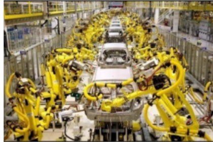
Figure 1 - Industrial robots enclosed from human interaction [3]
