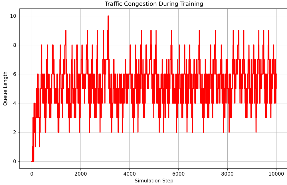
Figure 6.12: Queue length variation under DQN traffic signal control.
