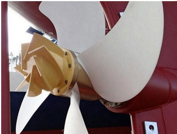
Figure 8: CFRP Blade Secured at the Hub (ClasNK, 2021)
