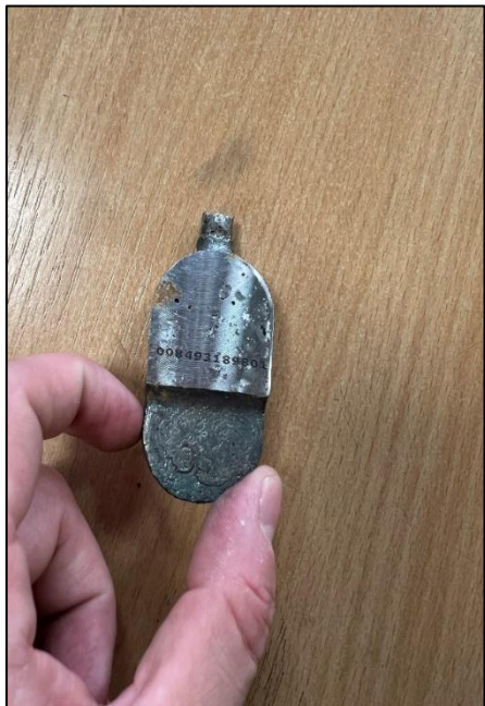
Figure 11 - Poorly Prepared Steel Sample
