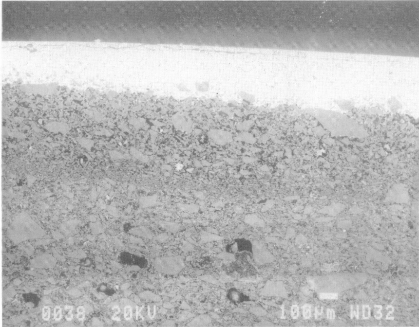
Plate 8 Backscattered electron micrograph of a polished section of a tile body and glaze from Bursa dated 1512–13 (Table 1, no.12). The multiple layers of ceramic raw materials (mainly silica) appear to be unnecessary: the second thin layer would be suitable as a slip but is sealed by the one overlaying it. This technology is quite obviously in ‘flux’, unlike the Iznik tile tradition (x50).
