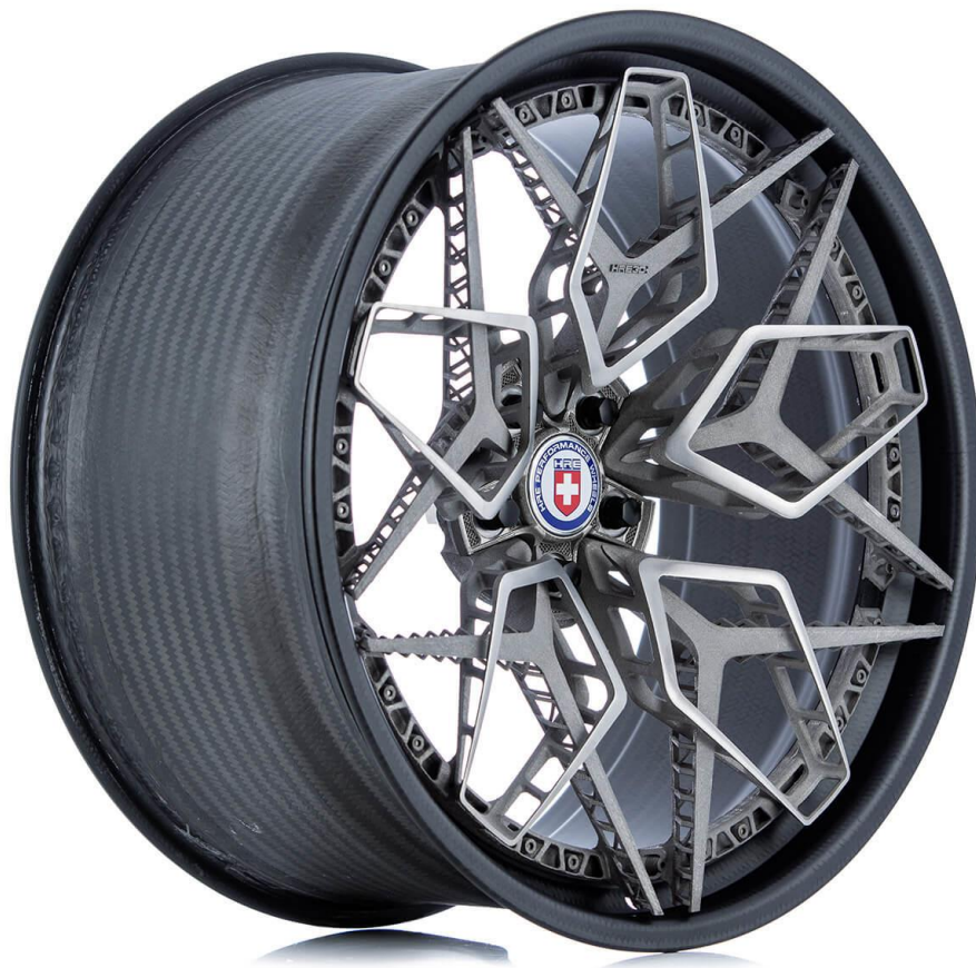
Figure 9 HRE 3d printed wheel (Source: HRE wheels.,2018: online)
