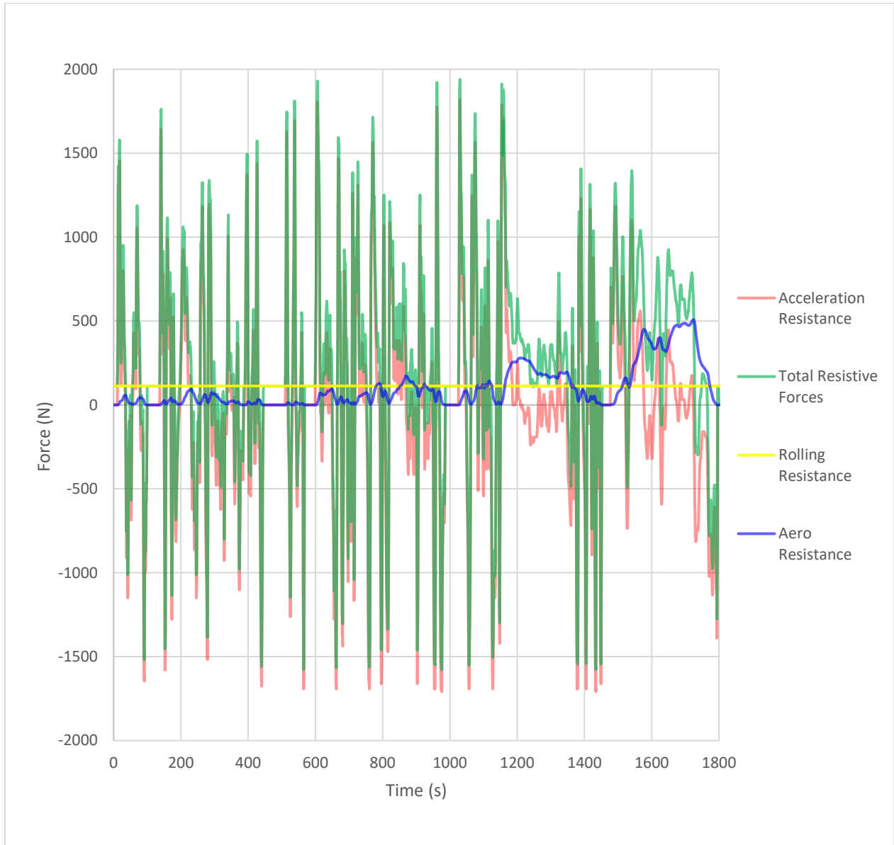
Figure 4 - Resistive Forces vs. Time Graph
