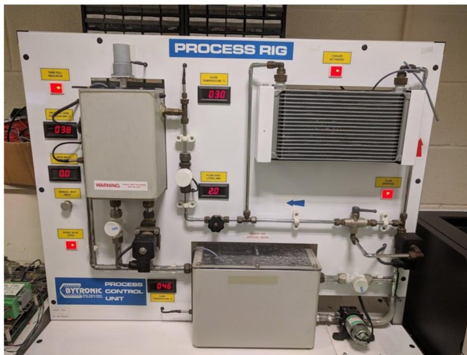
Figure 1 Bytronic Process Control Rig
