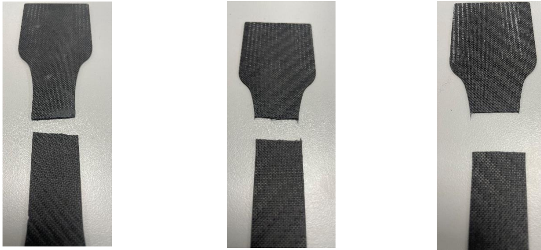
Figure 34: Carbon non-woven bio (left), Carbon woven bio (middle), Carbon woven epoxy (right)
