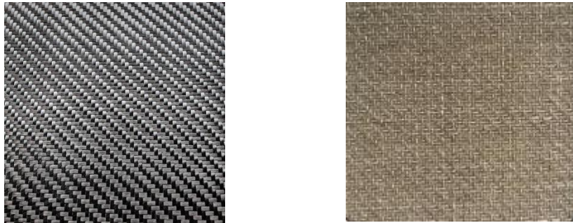
Figure 2: Carbon fibre taken from CarbonTouch, 2026 (left), Flax taken from EcoTechnilin, 2023a (right)
