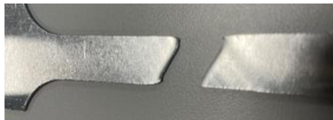
Figure 11: Coupon after test from present study
