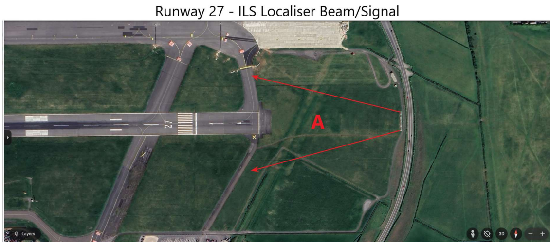
Figure 39 Runway 27 – ILS Localiser Signal (Google, 2024; Lewis, 2024)
