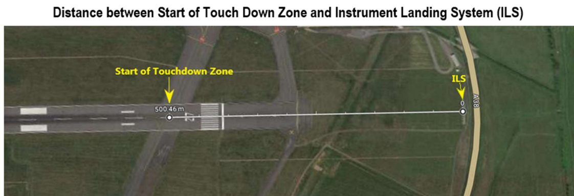
Figure 38 Distance between Start of Touchdown Zone and ILS (Google, 2024)
