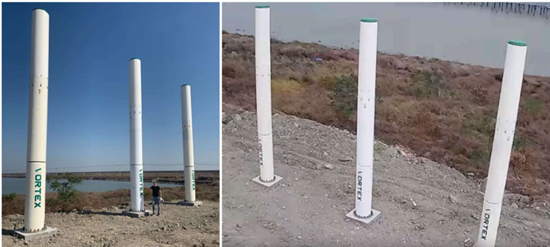
Figure 47 Vortex Bladeless Wind Turbines in Testing (Vortex, 2024)
