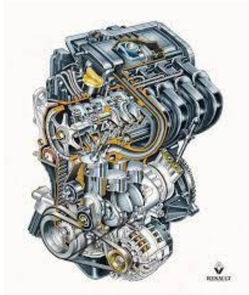
Figure 6 Above is a section view of the 1.2 Litre 16 valve Renault engine. (Renault, 2014)
