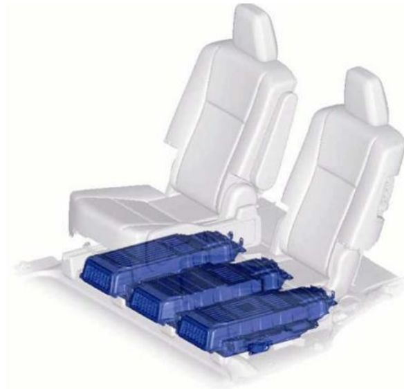
Figure 8: showing how the battery pack is located under the rear seats of the Toyota Highlander (Toyota Corporation, 2014)
