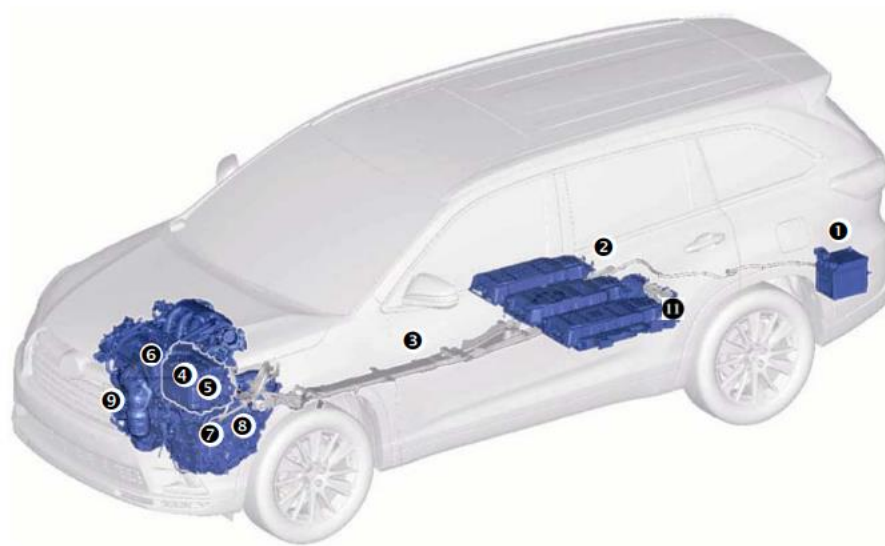
Figure 8: showing how the battery pack is located under the rear seats of the Toyota Highlander (Toyota Corporation, 2014)
