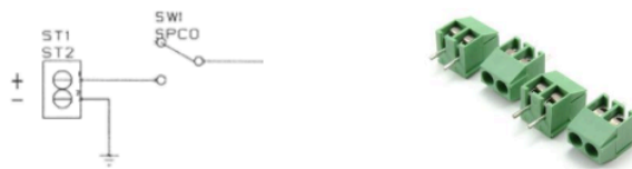
Fig 1.3. Screw Terminal in circuit and image of Screw Terminal
