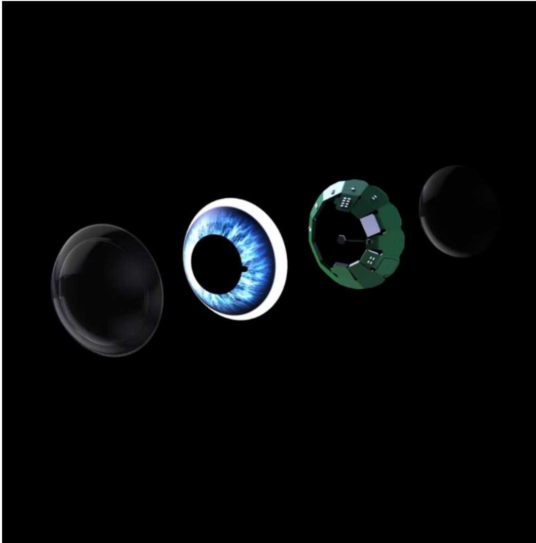
Figure Nine, Mojo scleral lens exploded view (Mojo Vision Inc, 2022)
