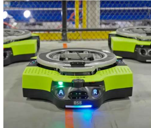
Proteus – Amazon's first collaborative ATV (Autonomous Transfer Vehicle), (Moon, 2022)
