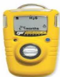
Figure 3 Example of H2S monitor worn by all personnel at the Pembroke plant
