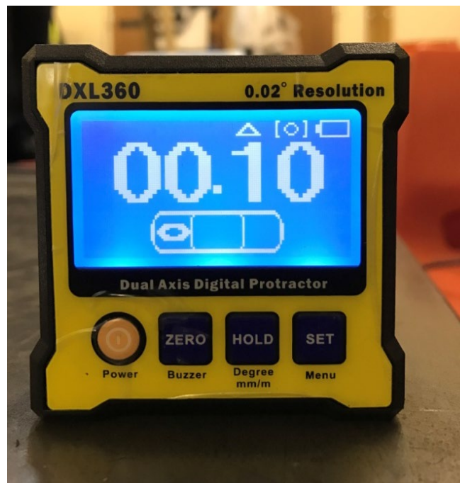
Figure 14: digital protector used for indoor measurements to determine the tilt angle.
