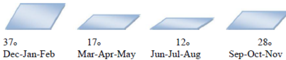
Figure 33: shows how the tilt angle is adjusted during a year in order to achieve the best performance (Chandrakar & Tiwari, 2013).
