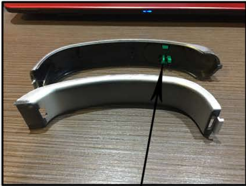
Handle & Switch (External) Material - Polystyrene (Thermoplastic Polymer) Assembly - Injection Moulding
