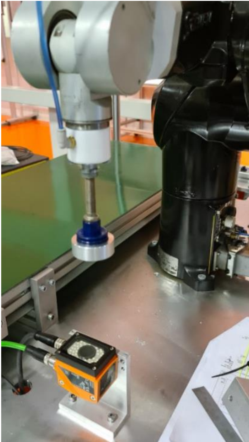
Figure 31 Camera location with robot holding part
