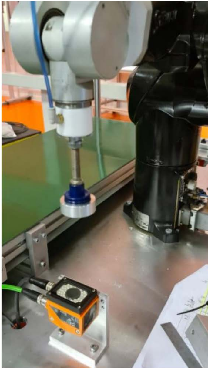
Figure 31 Camera location with robot holding part
