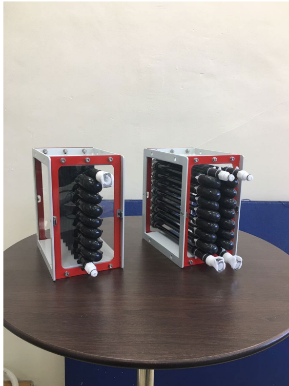
Figure 10 - Side by side 16 tube and 32 tube configuration
