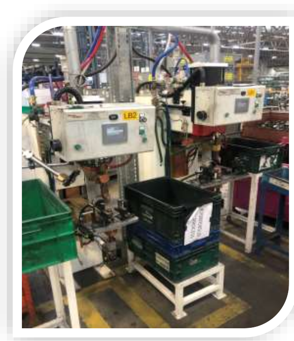
Figure 17 - 15.7170-02 M8 Stud and Nut Pedestal Welder
