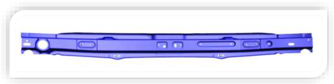
Figure 22 - 15.7661C Rear Bumper Beam with x2 M6 Nut Assembly
