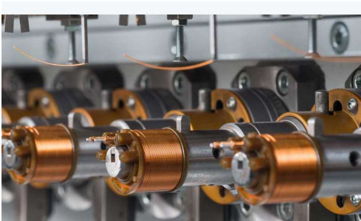
Image 4 – current production coil winding
