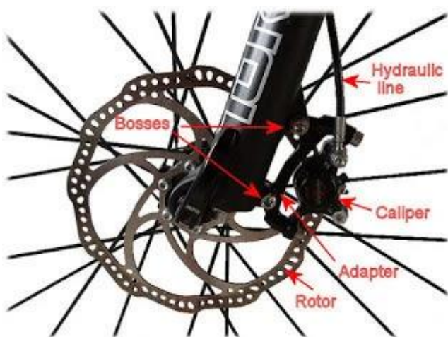
Figure 5:3:6 diagram showing how the soap box cars brake assembly works (Bicycle Disc Brakes, no date)
