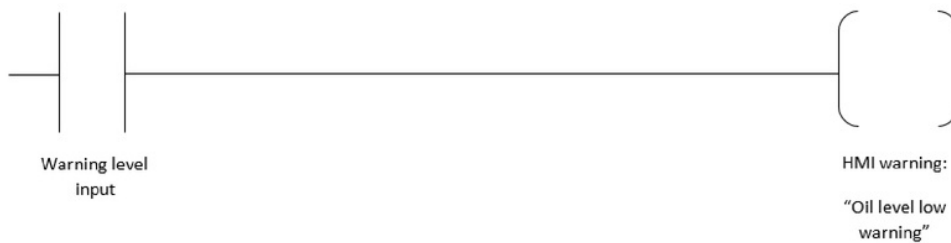
Figure 10: Warning input programming
