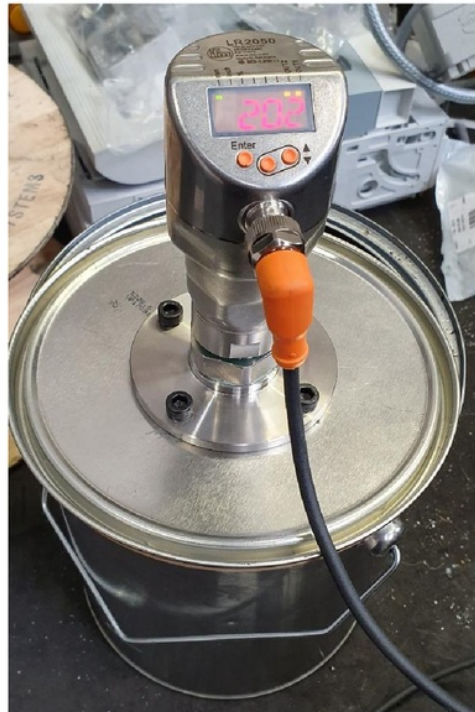
Figure 16: sensor readout on 80% full
