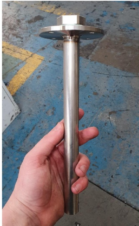
Figure 15: Flange plate with coaxial tube
