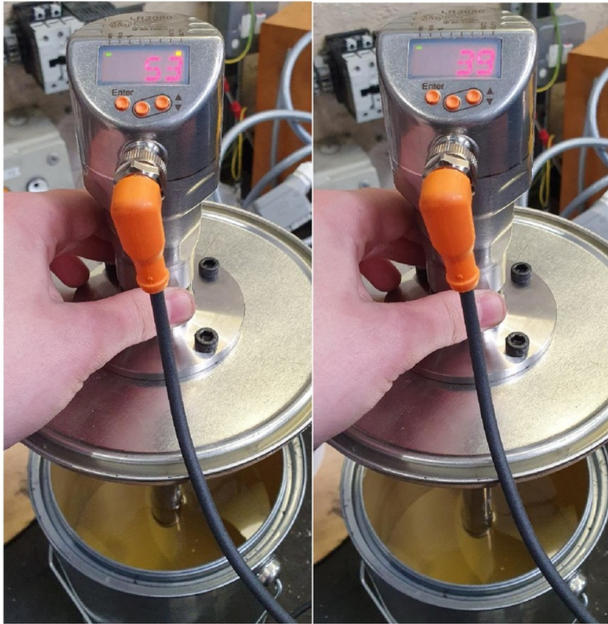
Figure 19: Level of sensor just above output 1 and when the level drops below 50mm
