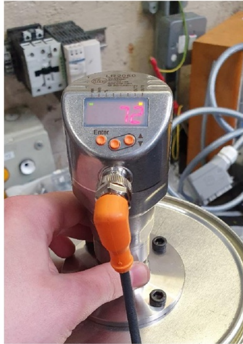
Figure 14: Sensor mounted to flange plate and mounted to lid
